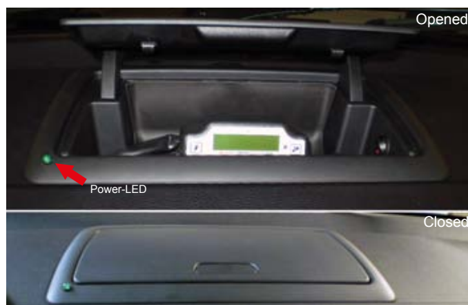
Stage 3 TD-Controller discreetly in the instrument panel compartment (BMW E82 123d)
