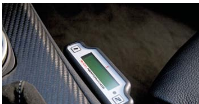
Mounting example: Stage 3 Controller between centre console and passenger seat (BMW E90)
