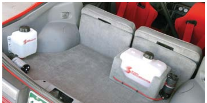
Mounting Example: 31 tank (separate brake cooling) and 9.5l trunk mounting kit with pump
